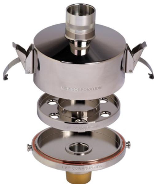
**Fig. 3.** NGI pre-separator; its single size-fractionating stage comprises six nozzles, each  $12.80 \pm 0.05$  mm in diameter [8]
